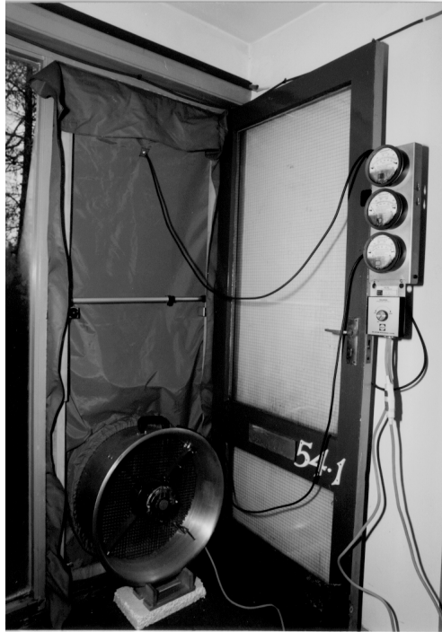
(a) Domestic Blower Door (Crown copyright - UK Building Research Establishment)
