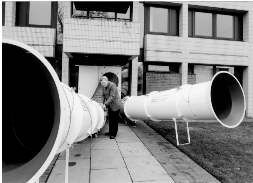
(b) Large Building Multi-fan System (Crown copyright - UK Building Research Establishment)
