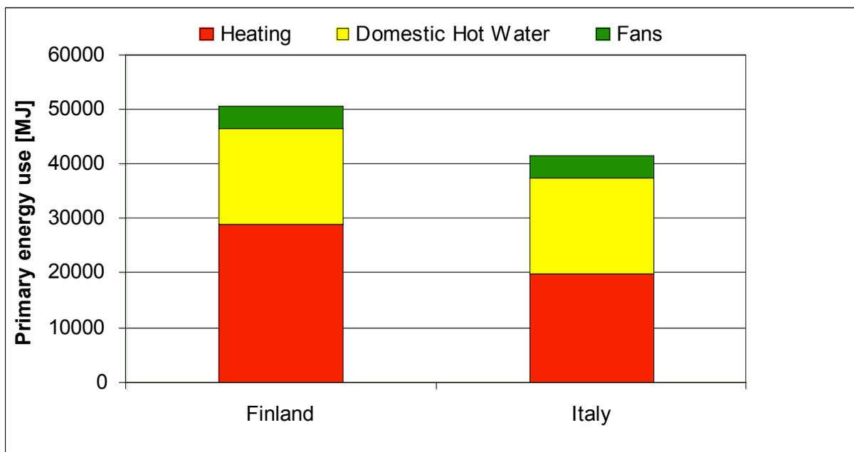
Figure 2: Energy use of the test house for the Finish set of energy saving measures and the Italian set of energy saving measures for a cold and hot climate respectively.
