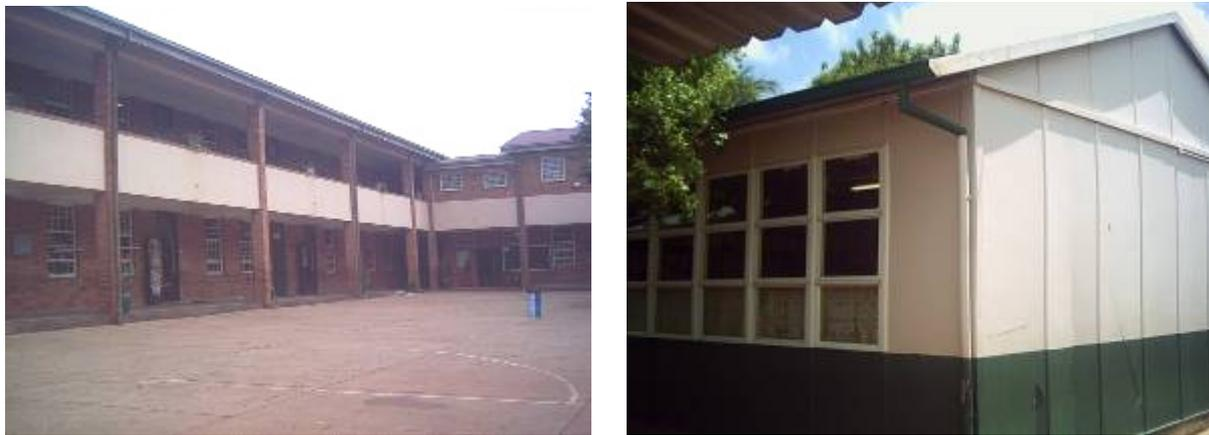
Figure 1: On the left: Emmarentia Primary School in Johannesburg with brick walls, concrete floors and balustrades and a corrugated iron roof. On the right: Prefabricated classroom at Laerskool Garsfontein in Tshwane.
