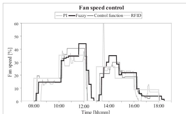
Figure 4: Time series evolution of the fan speed command
