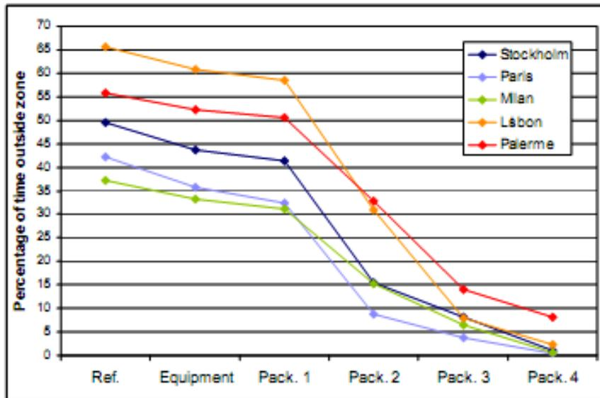
**Figure 2:** Reduction in discomfort index “percentage outside range” of EN15251.
