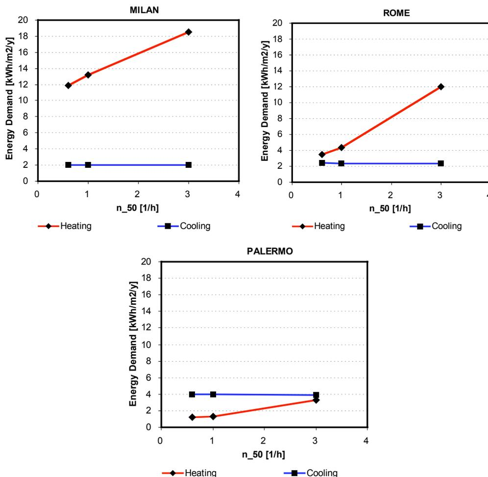
**Figure 1:** Winter and summer energy need for heating and cooling as a function of the building envelope air tightness (expressed by the  $n_{50}$  value).
