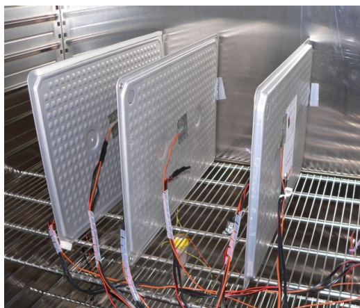
Figure 1: CSM panels in the environmental chamber
