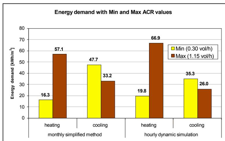
Figure 1: Thermal energy demand due to different air-change rates assessed by simplified and dynamic calculation methods.
