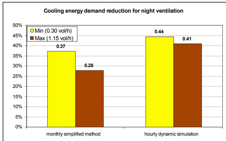
Figure 2: Cooling demand reduction with night ventilation strategy implementation.
