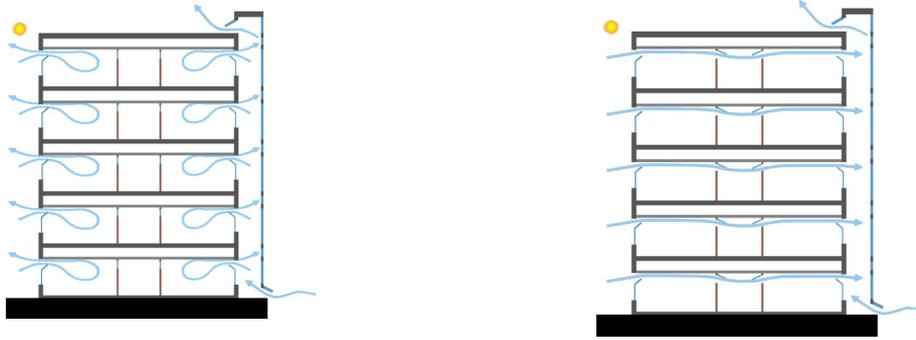
Figure 3. Offices with unilateral (left, simulation 3) and cross ventilation (right, simulation 4).
