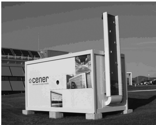
Figure 1: Solar chimney test rig.
