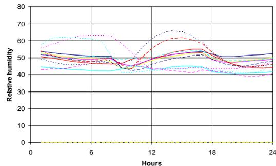
Figure 3: CE1B. Indoor relative humidity. Non-isothermal conditions and open surfaces. A day in July with solar and long wave radiation through the windows and on external opaque surfaces.
