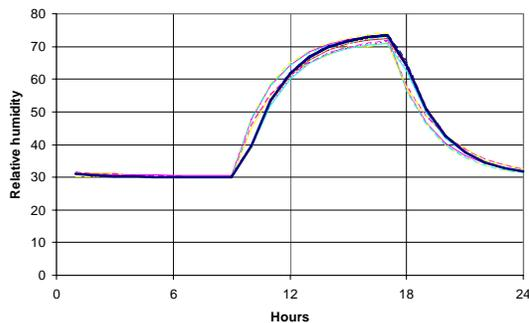
Figure 2: CE1A. Indoor relative humidity. Isothermal exposure. Construction surfaces are tight. The numerical results are compared with the analytical consensus solution.
