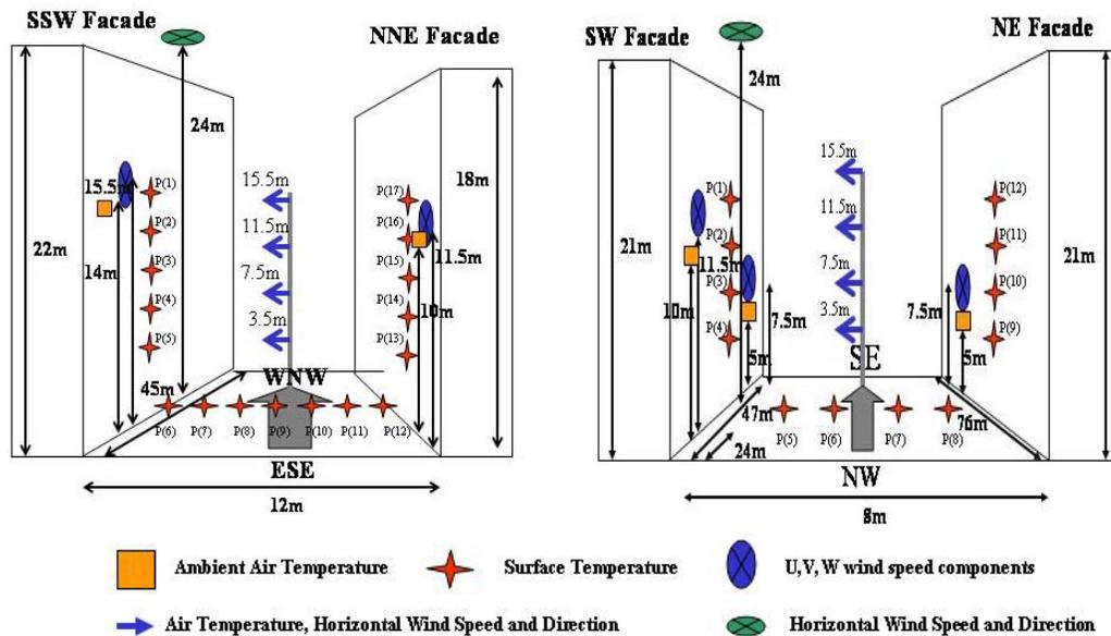
**Figure 1:** A schematic representation of the field measurements performed inside and outside the two urban street canyons (left is Ragavi and right is Ag. Fanouriou canyon)
