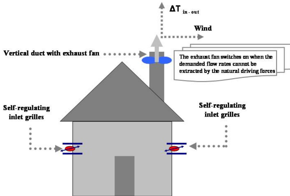
**Figure 5:** Representation of the RESHYVENT hybrid ventilation system for moderate climates
