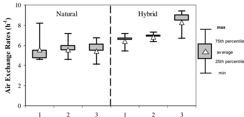
**Figure 3:** Boxplots of estimated air exchange rates (h<sup>-1</sup>) for natural (single-sided) and hybrid ventilation experiments at A<sub>3</sub> apartment, under calm conditions based on the single-zone (1,2) and multi-zone (3) methodologies
