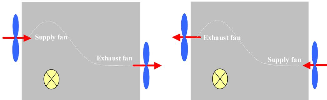
**Figure 4:** A representation of the pilot hybrid ventilation system with the two inlet/extract fans installed at the two external building walls. An inverse operation of the fans is considered on the right photo
