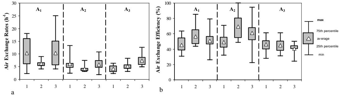
**Figure 2:** Boxplots of estimated air-exchange rates and air-exchange efficiency values (%) based on multi-zone method (h<sup>-1</sup>) for natural (1), mechanical (2) and hybrid (3) ventilation experiments under different ambient conditions
