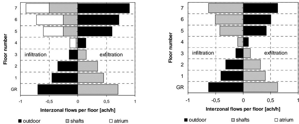
Figure 3. Flow balance per floor for moderate use of main entrances. Left: building with atrium above the 4<sup>th</sup> floor (existing case). Right: building without the atrium.
