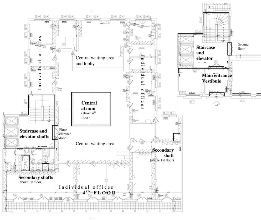
Figure 1. Left: Plan view of a representative floor of the examined building; upper right: main entrance and elevator shaft configuration in the ground floor. (Atrium, shafts and main entrances are highlighted)
