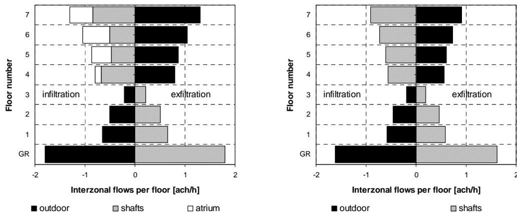
Figure 4. Flow balance per floor for peak-hours use of main entrances. Left: building with atrium above the 4<sup>th</sup> floor (existing case). Right: building without the atrium.
