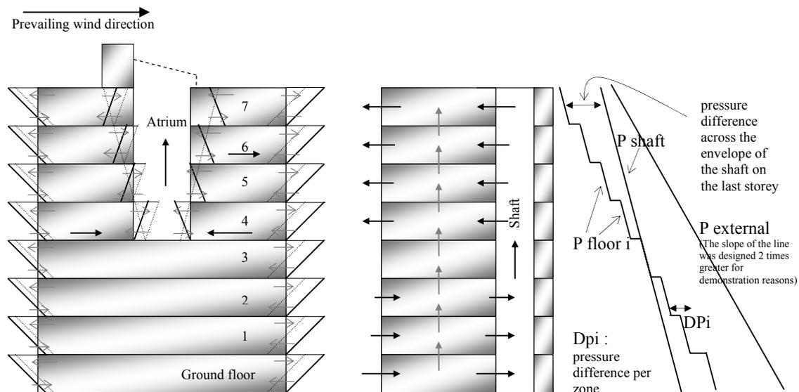
Figure 2. Pressure distribution and interzonal flows in the examined building; left: cross-section at the area of the atrium; middle: cross section at the area of the main shafts; right: internal and external pressure differences (slope lines)
