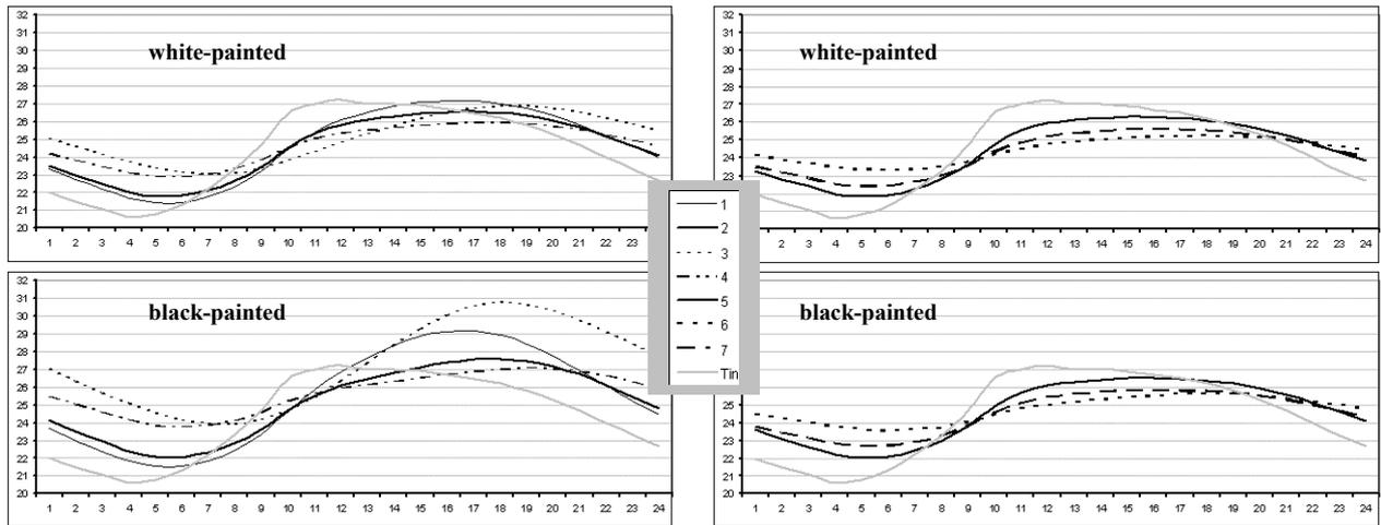
Figure 2: internal surface temperature for traditional (1-4) and retrofitted (5-7) walls
