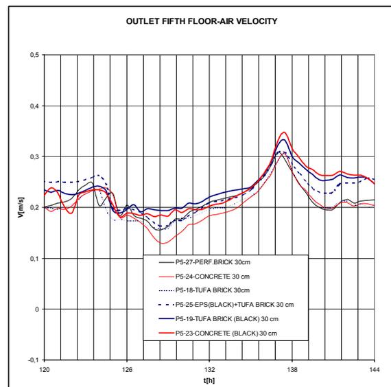
Figure 5: air velocity near the air-transfer device at the top of the entrance unit (grilles at the first and fifth floors).
