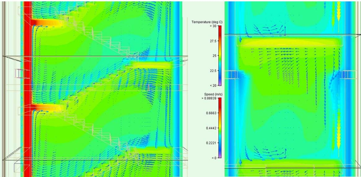
Figure 4: details of fluid flow and temperatures at the first floor (longitudinal and cross section). Case 3 (black-painted) at 04:30h (above) and at 17:00h (below).
