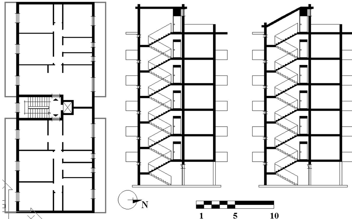
Figure 1: the adopted model: typical plan and section
