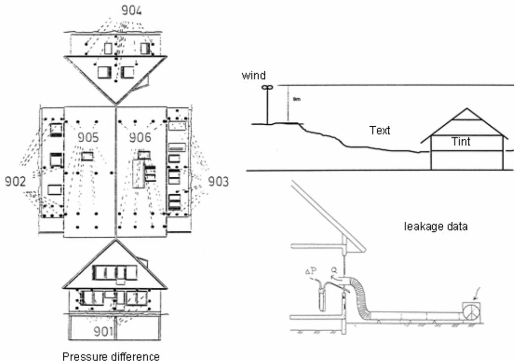
Figure 2. Measurement program for validation of probabilistic model of air infiltration
