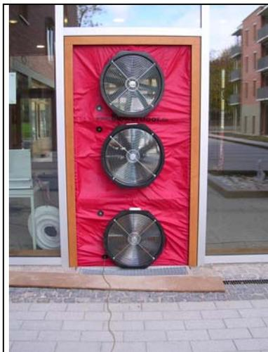
Figure 2: External view, installation of 3 blower door units in one external door
