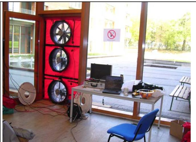
Figure 3: Internal view; aluminium frame with 2 middle cross bars; 3 blower door units (open, without reducing rings); APT 8 - Automated Performance Testing system in case; notebook with TECLOG and BlowerDoor plus
