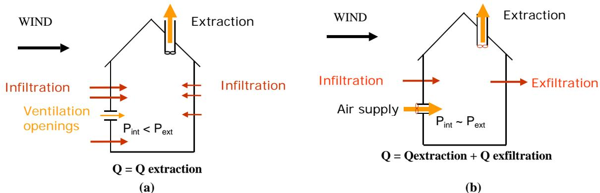
**Figure 1 : Influence of the ventilation system on the total air change rate of a building. Case of a good airtightness : (a) building ventilated with an extract ventilation system, (b) : building ventilated with a supply-extract ventilation system.**
