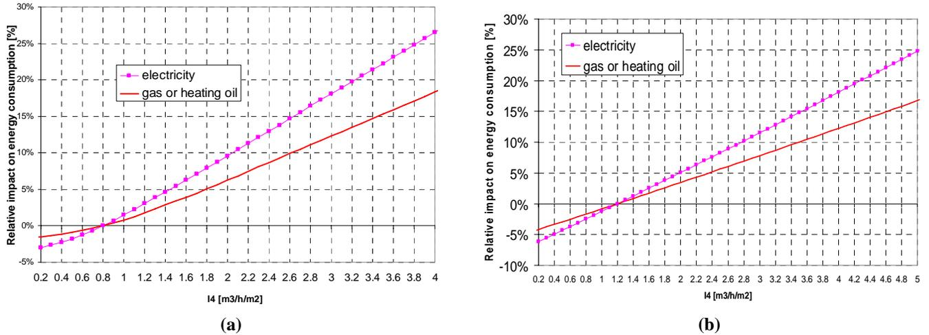
**Figure 3 : Influence of the building envelope air-tightness on the total energy consumption. (a): single family dwelling ventilated with an extract ventilation system, simulation file : CSTB file MI4 THC-APP-04 ref.thc, (b): office building ventilated with a supply-extract ventilation system without heat exchanger, simulation file : CSTB file bureaux2 THC-APP-14 ref.thc.**
