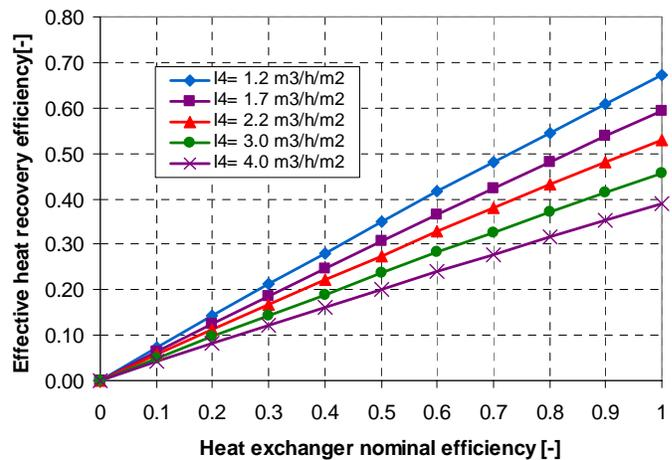
**Figure 5 : Influence of the building air-tightness on the effective heat recovery for an office building ventilated with a supply-extract ventilation system. Sim. file : CSTB file bureaux2 THC-APP-14 ref.thc.**
