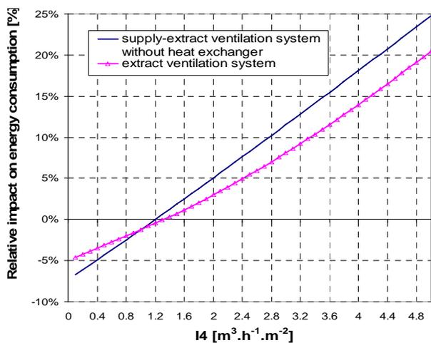
**Figure 4 : Influence of the building air-tightness for an office building ventilated respectively with an extract – and a supply extract system. Sim. file : CSTB file bureaux2 THC-APP-14 ref.thc.**
