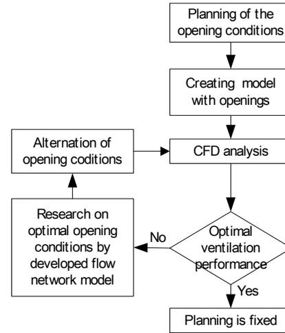
Figure 2. Flow chart for planning by CFD and developed flow network model analysis
