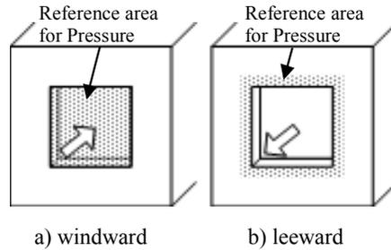
Figure 6. Reference area for pressure coefficient
