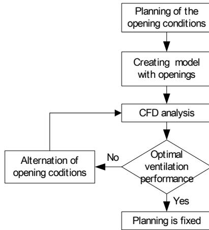
Figure 1. Flow chart for planning by only CFD
