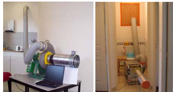
Figure 1. IMPEC onsite measurement protocols: connected to the mechanical ventilation network (left) or to a wooden “fake trap” (right)
