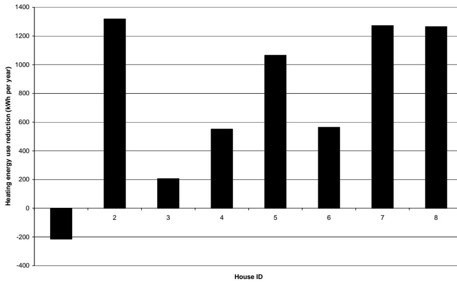
Figure 4. Estimates of heating energy use reduction on a heating season ( 2500 degree days).
