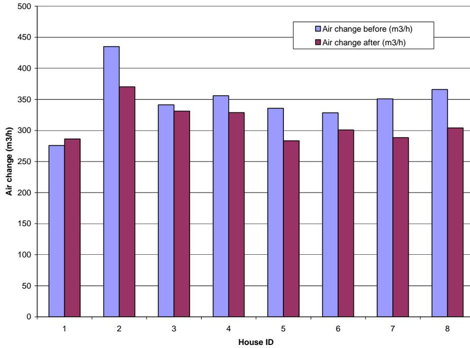
Figure 3. Estimates of air change rate before and after refurbishment.
