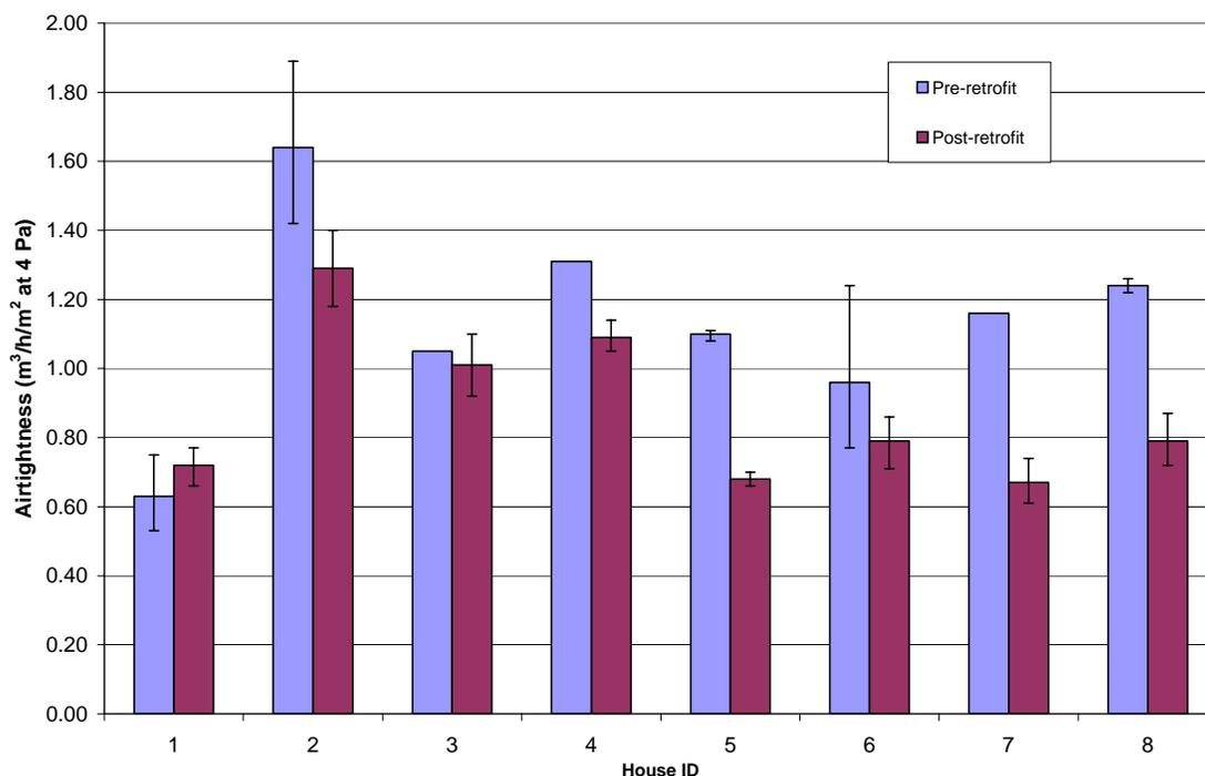
Figure 2. Pre- and post- airtightness measurements in  $\text{m}^3/\text{h}$  per  $\text{m}^2$  of cold walls (except lower floor) at 4 Pa.
