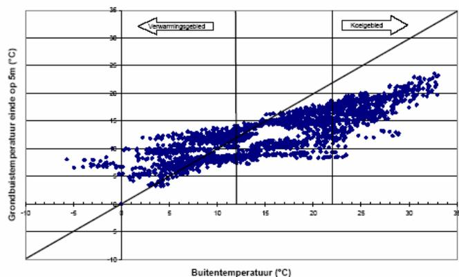
Figure 2: Measured outlet vs inlet EAHX temperature
