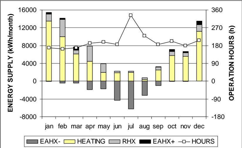
Figure 4: Measured energy supply (Desmedt et al. 2004)
