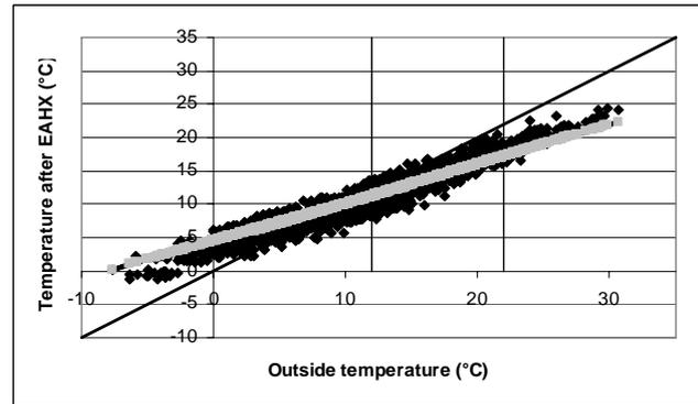
Figure 6: Predicted outlet vs inlet EAHX temperature
