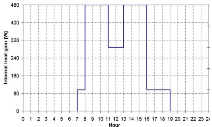
Figure 2: Schedule of the internal heat gain
