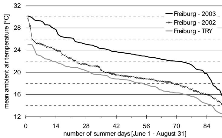
Figure 6: Comparison of ambient air temperature for the summer 2003 and the test reference year TRY 7. The summer 2002 was a typical summer. Obviously, the TRY 7 does not consider high ambient air temperatures. The summer 2003 was 5.2 K warmer than the design weather TRY 7 with long periods of warm weather.
