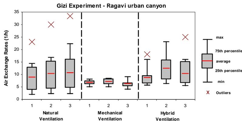
**Figure 8.** Estimated air exchange rates (1/h) for the total number of ventilation experiments.
