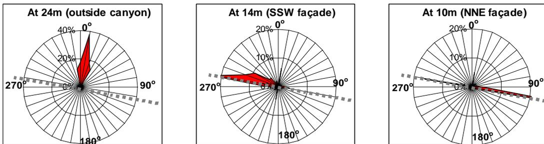
**Figure 6.** Horizontal wind direction outside canyon and near canyon façades, when the ambient wind comes from northern directions ( $10^{\circ}\pm 20^{\circ}$ ).
