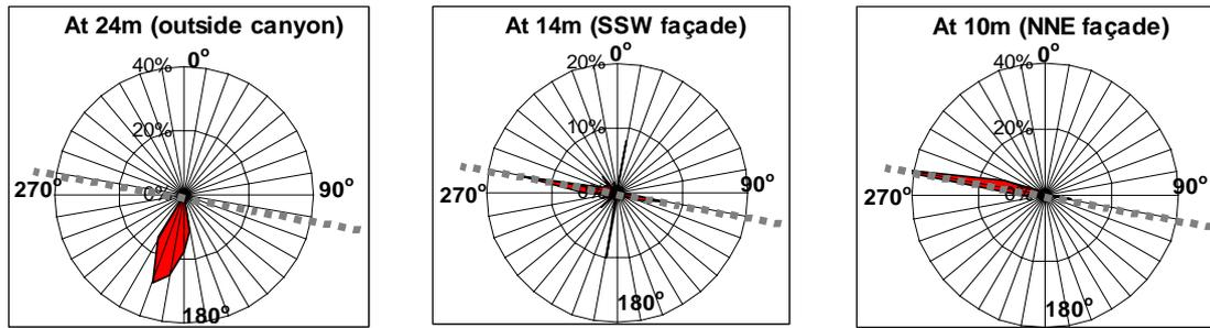
**Figure 5.** Horizontal wind direction outside canyon and near canyon façades, when the ambient wind comes from southern directions ( $190^{\circ}\pm 20^{\circ}$ ).
