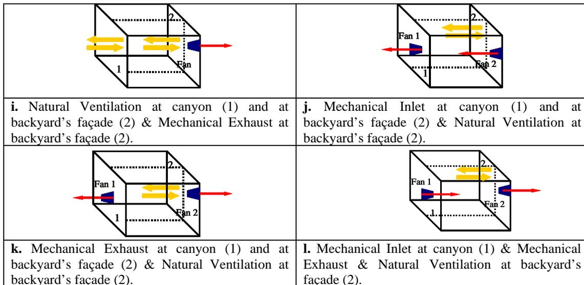
**Figure 3.** The hybrid ventilation systems studied at the ventilation experiments in the three dwellings during summer 2002 in Athens.
