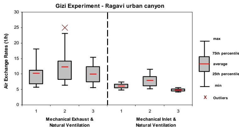
**Figure 9.** Estimated air exchange rates (1/h) for the hybrid ventilation experiments.
