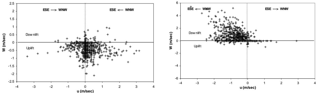
**Figure 7.** Along canyon wind speed,  $u$ , against vertical wind speed,  $w$ , near a) SSW and b) NNE façade, when the incidence angle of the ambient wind is perpendicular to the canyon axis from southern directions ( $190^\circ \pm 20^\circ$ ).
