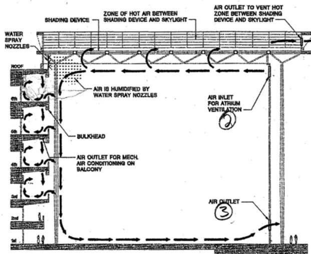
Figure 10: Diagrammatic description of air flow.
