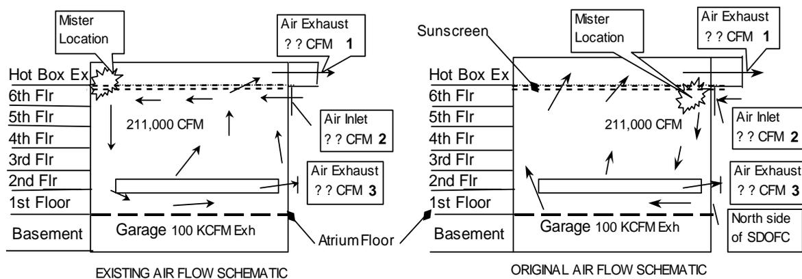
Figure 1: The Atrium's Existing and Original Air Flow Schematics
