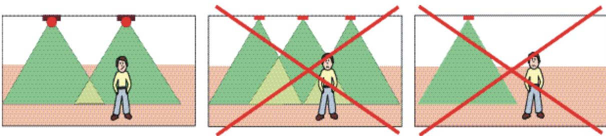
Figure 1 : correct position of infrared sensors in the room
