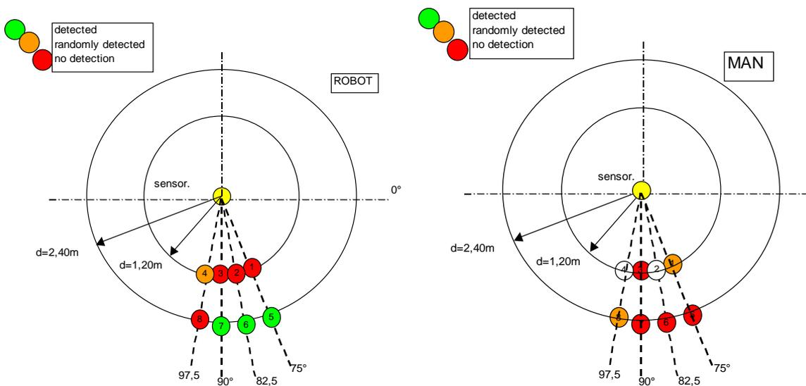
Figure 5 : example of detection by robot on another sensor, and comparison with a detection with man movement
