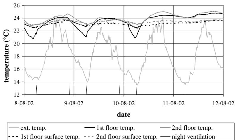
Figure 2: operation of natural night ventilation
