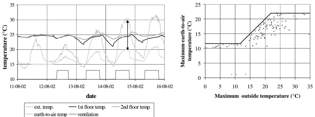
Figure 3: earth-to-air heat exchanger: operation (left) and cooling effect (right) (De Paepe, 2003)
