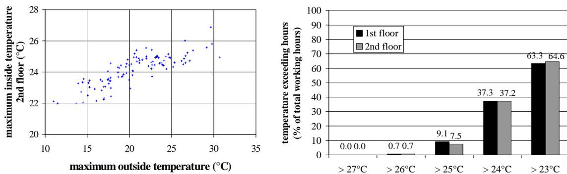
Figure 6: Maximum air temperature at 2nd floor as a function of the maximum outside air temperature (left) and temperature exceeding hours at both floors (right) from May 15 to September 30, 2002 (TRY Ukkel)
