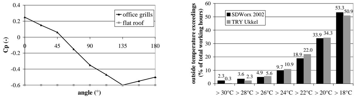
Figure 5: Wind surface pressure coefficient  $C_p$  varies with the angle between the wind direction and the normal on the surface (Orme et al., 1994) (left) and Weather data (May 15 till September 30): comparison outside temperatures exceedings on site - Test Reference Year Ukkel
