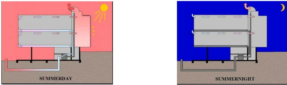
Figure 1: Operation of passive cooling: earth-to-air heat exchanger and ventilation by day (left) and natural night ventilation (right) (Cenergie, 2002)
