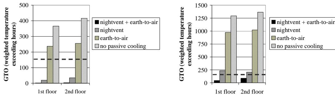
Figure 7: Weighted temperature exceeding hours (GTO) from May 15 to September 30, 2002 (TRY Ukkel) at current (left) and maximum occupation (right)
