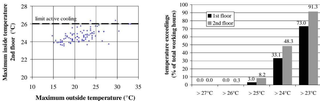
Figure 4: Maximum inside temperature at 2nd floor as a function of the maximum outside temperature (left) and temperature exceeding hours at both floors (right) from May 15 to September 30, 2002 (De Paepe, 2003)
