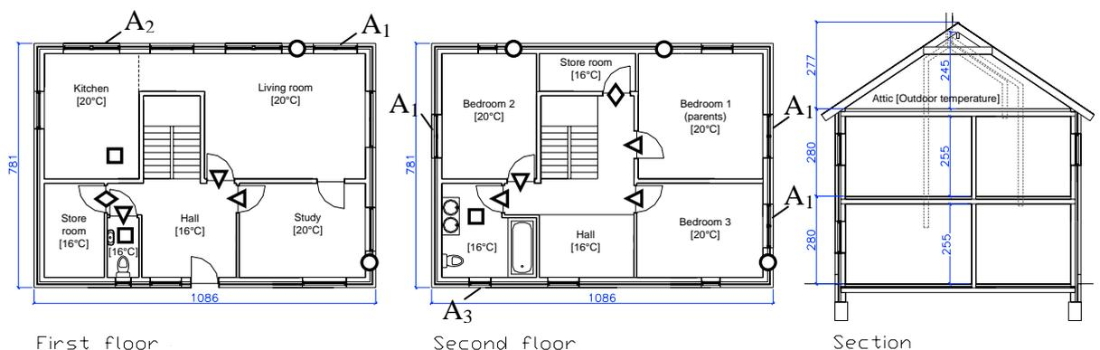
○ = ventilation inlet    □ = ventilation outlet (vertical duct)    △ = transfer opening    ◇ = store room ventilation
