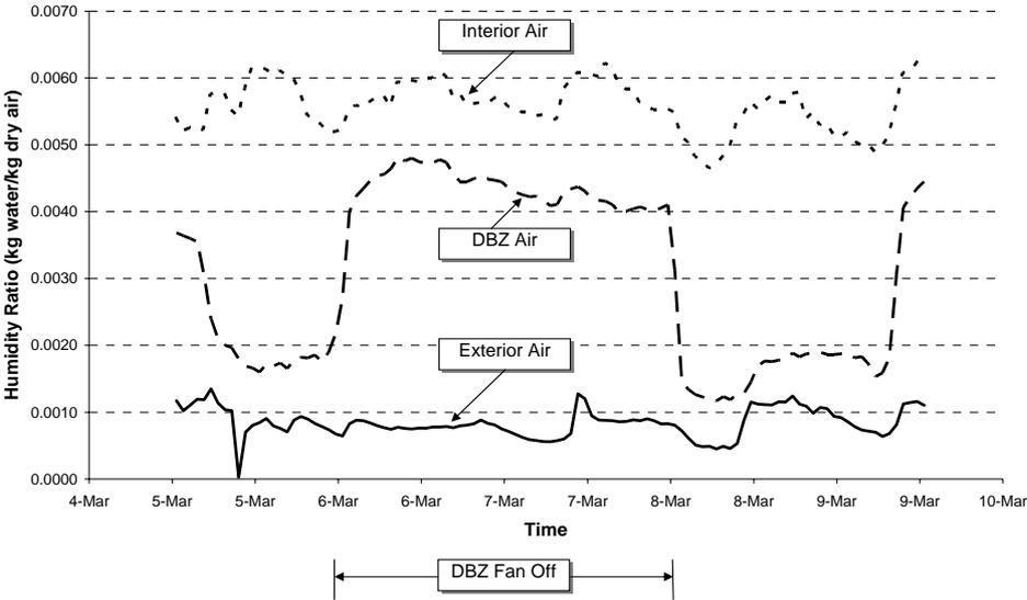
Figure 3 - DBZ monitoring results for the thirteenth floor.
