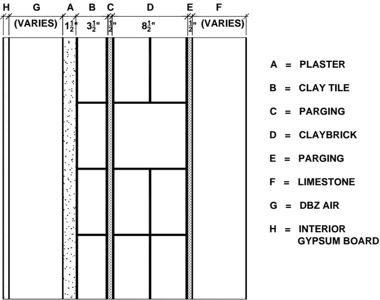
Figure 2 - General wall configuration incorporating the DBZ. Note that many different wall conditions existed.
