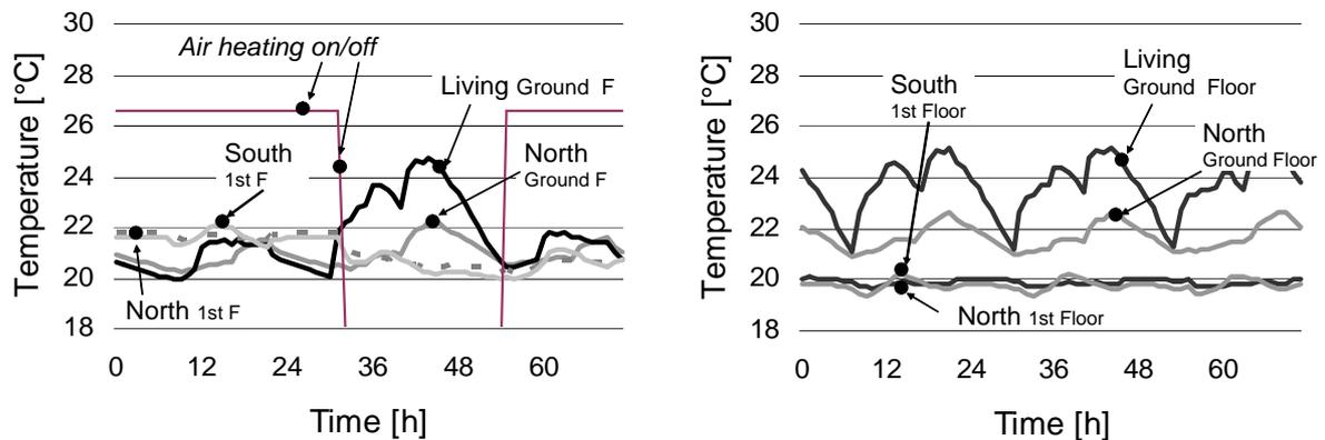
Figure 7: Room air temperatures with internal doors open. Stove fired twice a day (morning and evening) during one specific day; air heating the days before and afterward (left). Stove fired twice a day (morning and evening) during a series of days (right)
