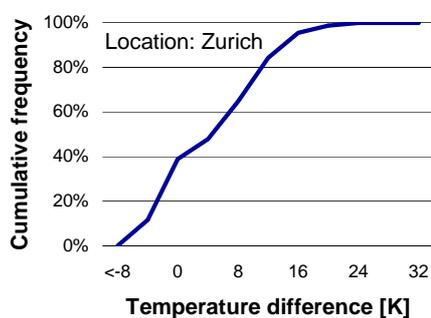
Figure 1: Cumulative frequency of the temperature difference between supply air and living room air temperature. Time period October to March for moderate climate (Zurich, Switzerland)
