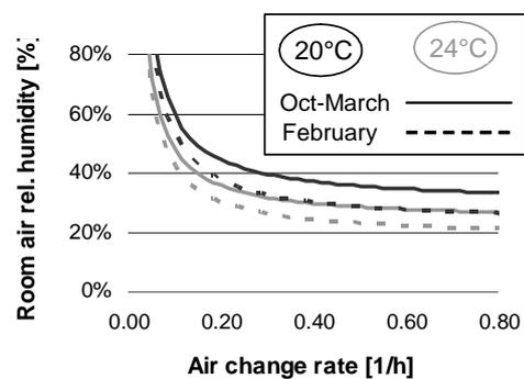
Figure 2: Room air relative humidity (steady state) as a function of outdoor air change rate, for two indoor temperatures and two typical winter periods. Living area 60 m<sup>2</sup>/person
