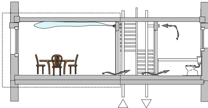
Figure 3: Typical Passive House ventilation configuration with far throw jet air inlet positioned at the internal wall to the corridor. The space covered by measurements is indicated by dotted lines
