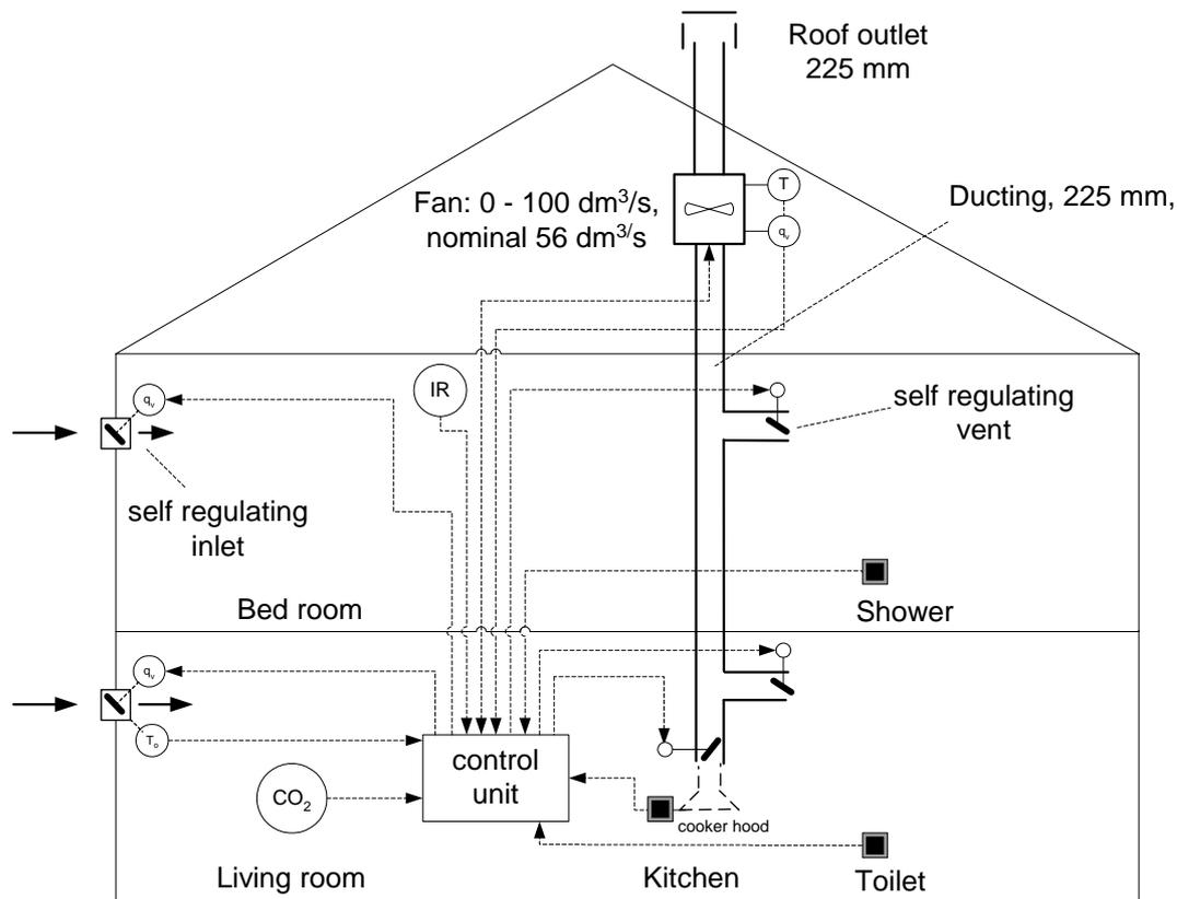
Figure 1: demand controlled hybrid ventilation system in family house.
