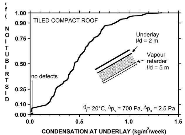
FIGURE 2: Predicted distribution of condensation amount at underlay surface (surface-averaged value)
