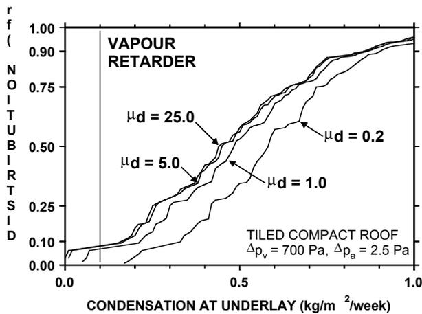
FIGURE 5: Effect of diffusion thickness of vapour retarder on condensation amounts at underlay surface
