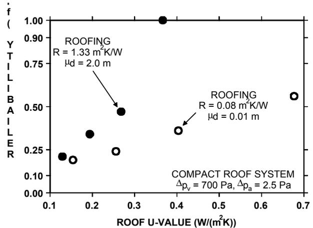
FIGURE 6: Effect of roof thermal quality on condensation control reliability
