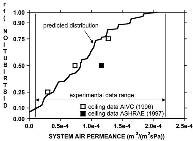
FIGURE 1: Comparison between predicted distribution and experimental data of system air permeance
