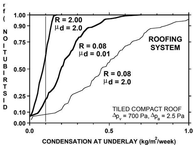
FIGURE 3: Effect of vapour permeable or thermally insulating roofing system on condensation at underlay
