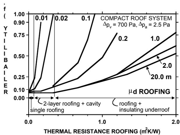
FIGURE 4: Combined effect of vapour permeable and insulating roofing systems on system reliability
