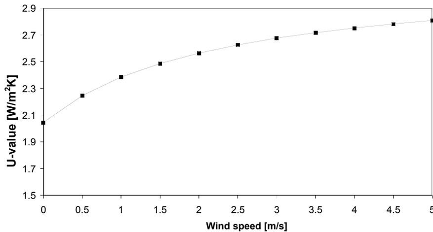
Figure 5: the theoretical variation of double glazing U-value with wind speed.
