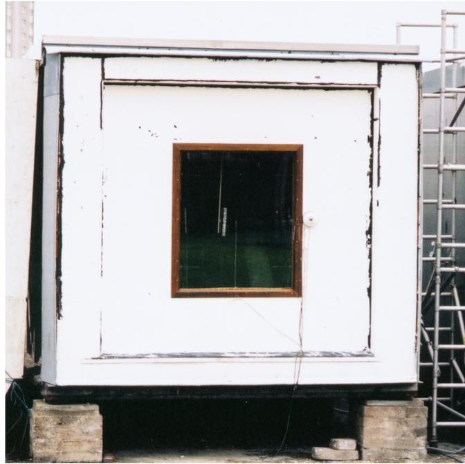
Figure 2: The window installed in the opaque surround at BRE Scotland.
