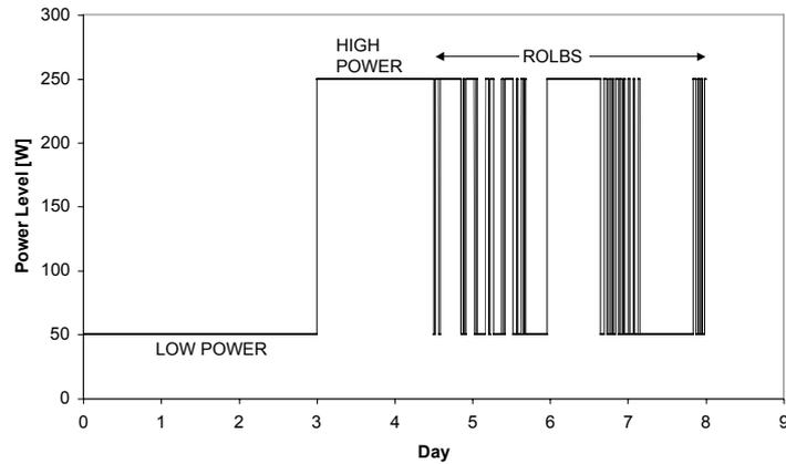
Figure 3: a typical heating power sequence with low power = 50W air circulation fan; high power = 50W fan power + 200W resistance heater.
