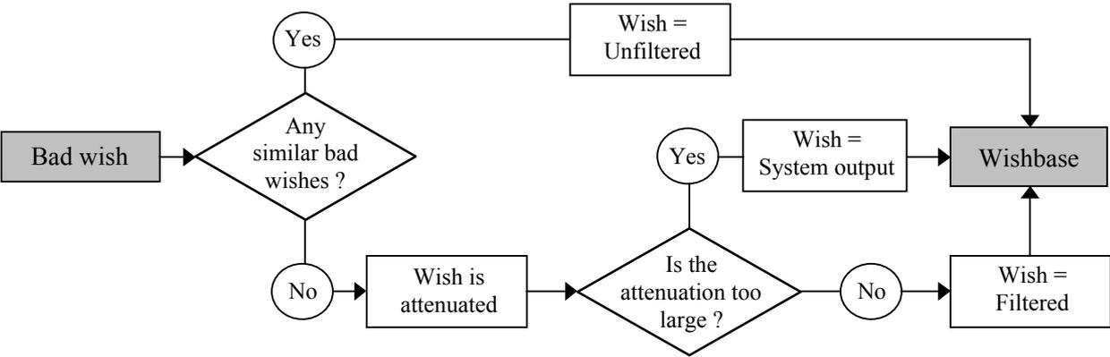
Figure 1: Operation diagram of the “wish pre-processing filter”. This filter is applied when the wish is detected as being bad from an energetic point of view.
