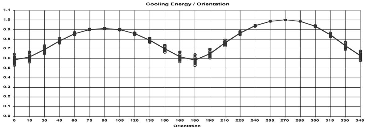
Figure 2. Energy necessary to cool the offices for various building orientations
