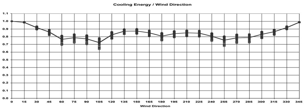
Figure 3. Energy necessary to cool the offices for various wind directions
