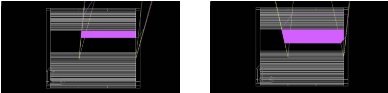
Figure 11 : Electrochromic protection (colored state) – work plan protected on June 21 from 3pm to 4pm.
