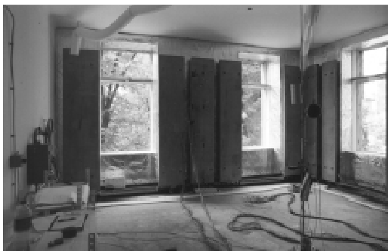
Fig. 4: View of heating-cooling concrete panells in experimental room.
