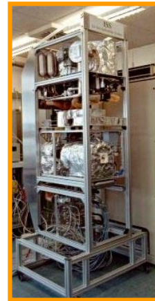
Figure 11: Closed Loop Air System Revitalization System Demonstrator
