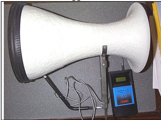
Cone, for air flow measurement (with anemometer)
