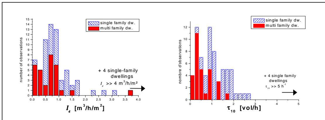
**Figure 7** Airtightness performance of buildings as a function of construction types.
