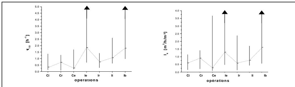
**Figure 8** Range and median values of airtightness indicators as a function of construction types.
