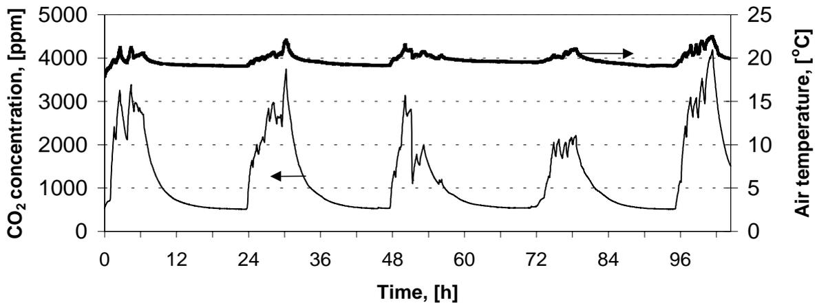
Fig. 1. Variability of carbon dioxide concentration and air temperature, in one of examined classrooms.
