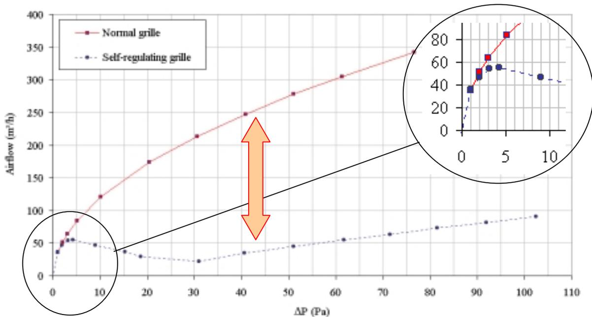
**Figure 7: Measured characteristic of the self-regulating grille used per meter length**
