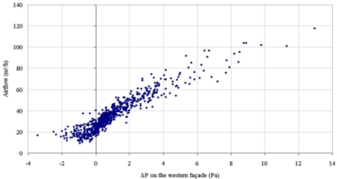
**Figure 4: Correlation between airflow measured in the small bedroom and the difference of pressure on the façade where the supply grille is installed**
