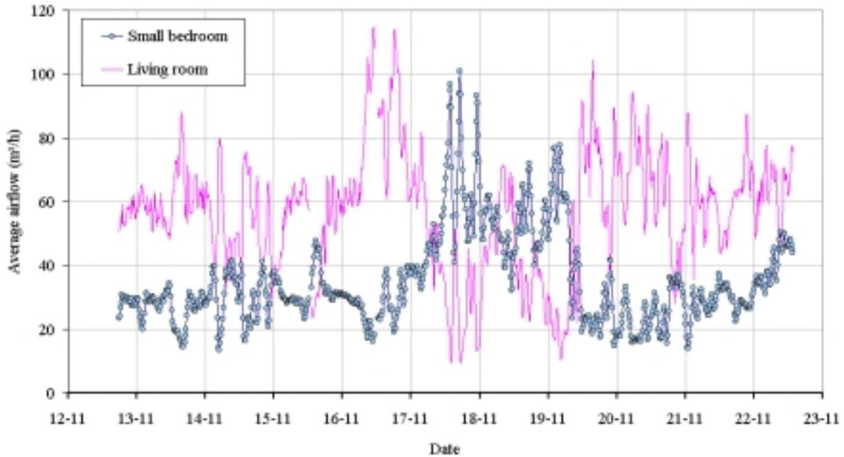
**Figure 3: Airflows measured in rooms equipped with natural supply grilles**
