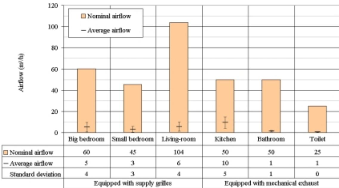
**Figure 11: Airflows observed when no ventilation system is used**
