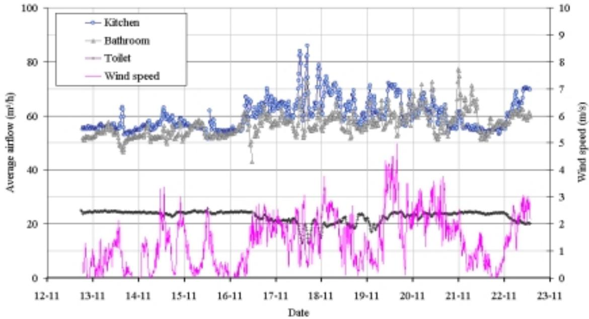
Figure 5: Airflows measured in rooms equipped with permanent mechanical exhaust
