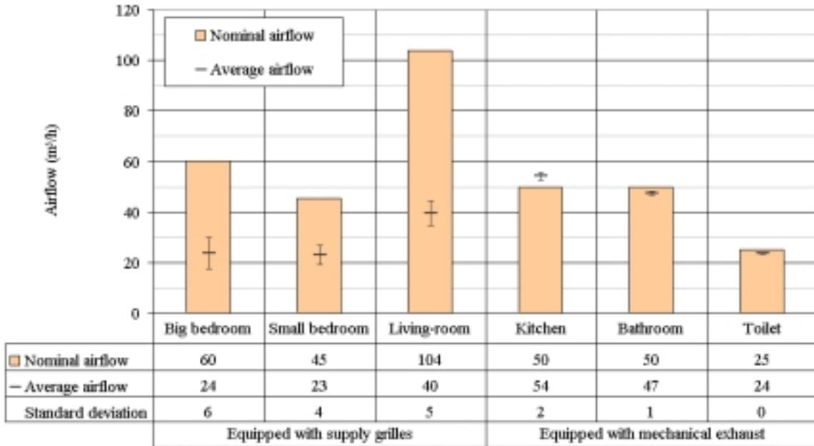
**Figure 10: Summary of the airflows measured with the supply grilles closed**
