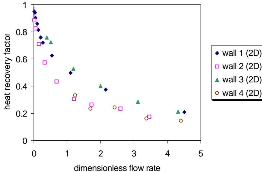
Figure 3: Heat recovery factor determined from 2D CFD simulations for walls 1-4. Solid symbols show data for walls with a high/low hole configuration (1 and 3) and hollow symbols show data for walls with a straight through hole configuration (2 and 4). Notice the two distinct trends—one for each hole configuration.
