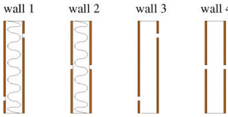
Figure 2: Wall geometries 1-4; 1 & 2 are insulated and 3 & 4 are empty.
