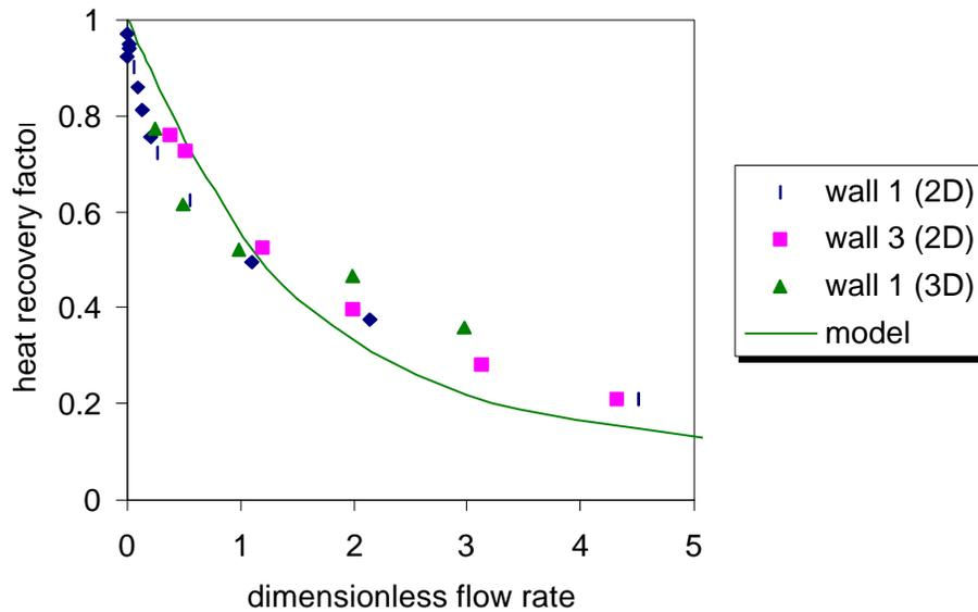
Figure 5: Heat recovery factor for walls with a high/low hole configuration (insulated and empty wall cavities) determined from CFD simulations and the simplified model using a constant area ratio ( $f=0.33$ ).
