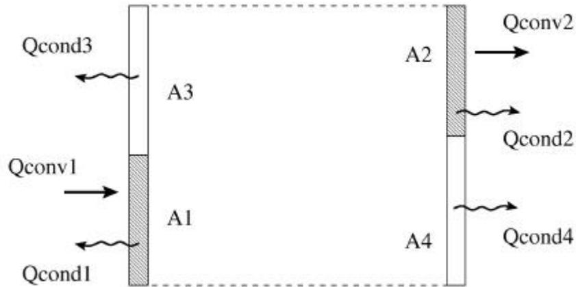
Figure 4: Energy flux through the simplified building envelope used in the model development. Sections A1 and A2 are affected by leaking air and have both convection and conduction terms. Sections A3 and A4 are not affected and have only a conduction term. The outer faces of the left and right walls form the system control volume boundary.
