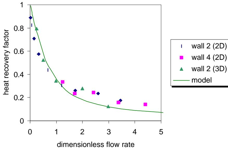
Figure 6: Heat recovery factor for walls with a straight through hole configuration (insulated and empty wall cavities) determined from CFD simulations and the analytical model using a constant area ratio ( $f=0.18$ ).
