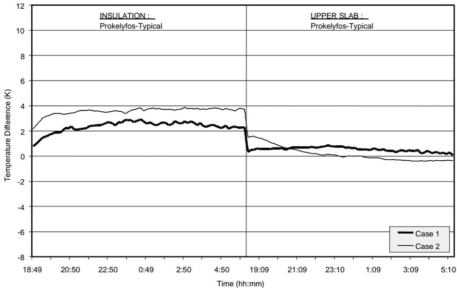
Figure 6. Nighttime temperature differences between the Ventilated and Typical components.
