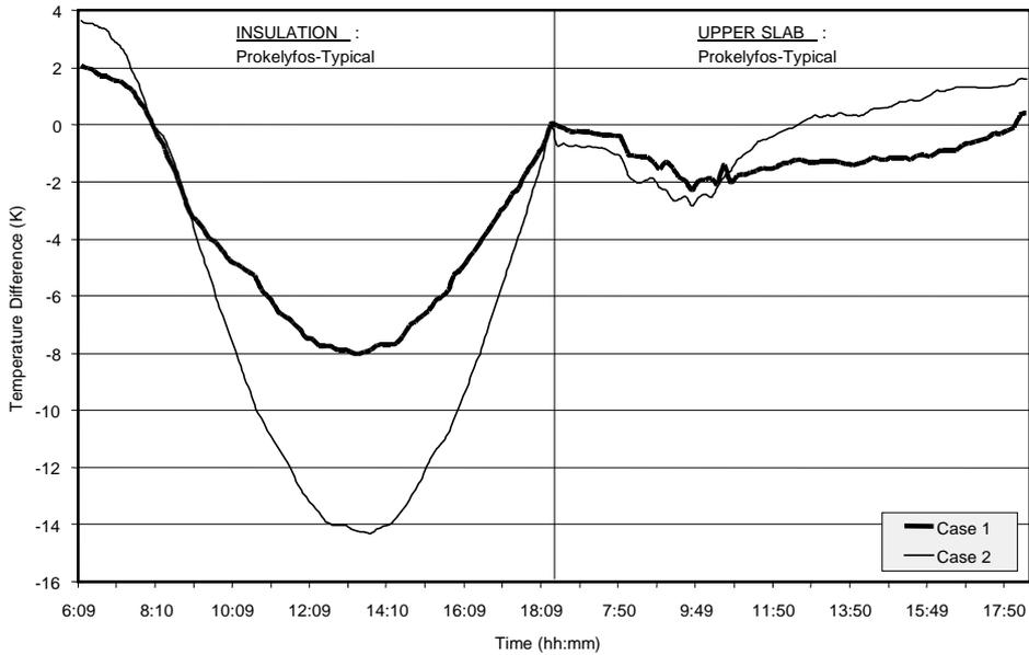
Figure 5. Daily temperature differences between the Ventilated and Typical roof components.
