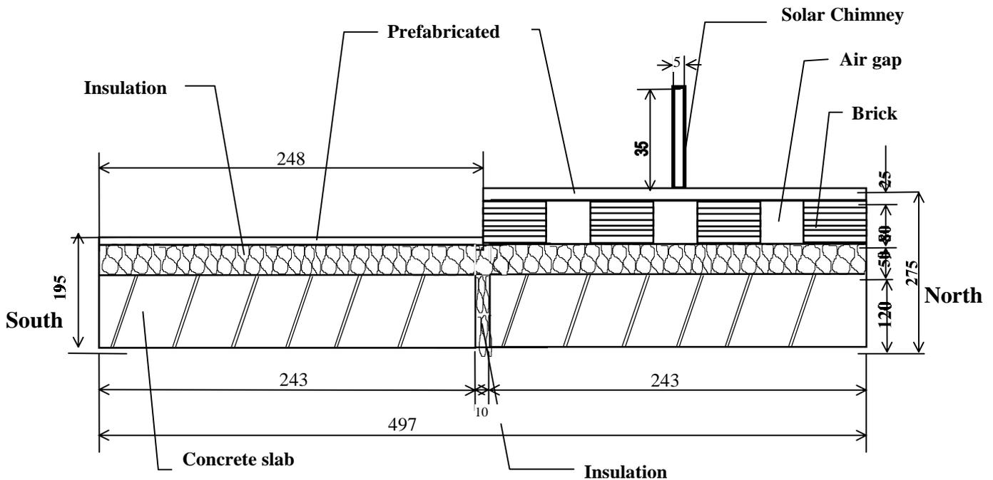
Figure 1. Cross-section of the roof components (not to scale).
