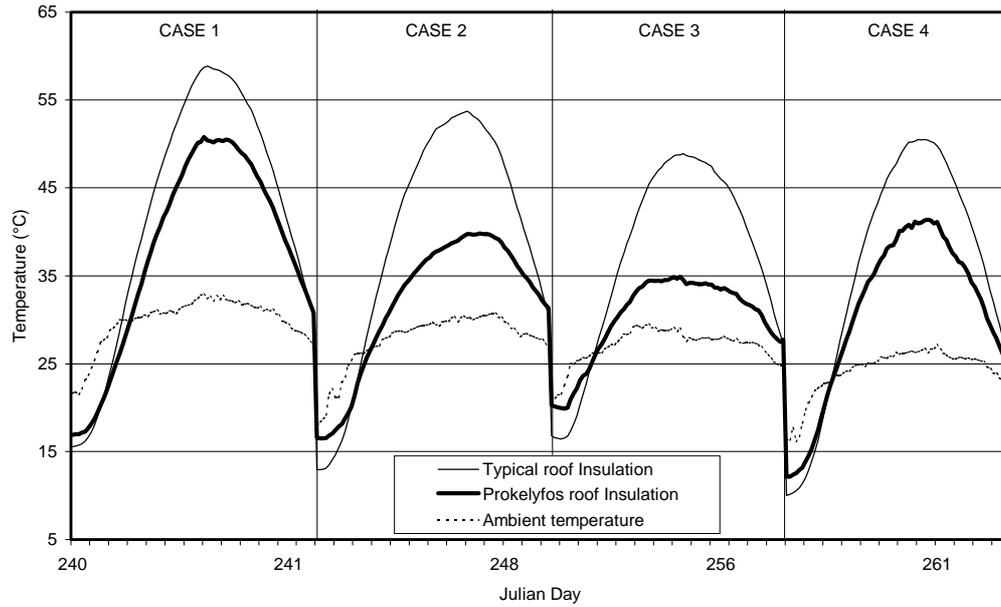
Figure 3. Daytime, temperature distribution of the Typical and Ventilated roofs insulation upper surface.
