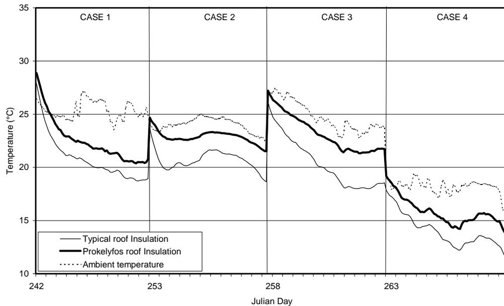
Figure 4. Nighttime temperature distribution of the Typical and Ventilated roofs insulation upper surface.
