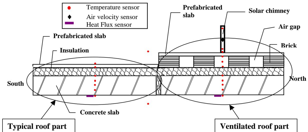
Figure 2. Sensor positions on the roof component.
