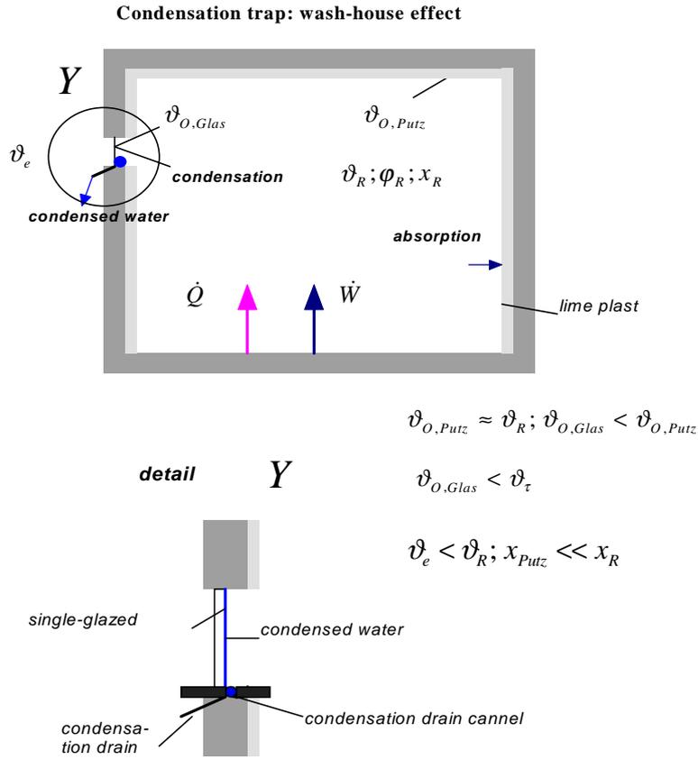
**Fig. 3:** Schematic representation of a condensation trap in a "wash-house"
