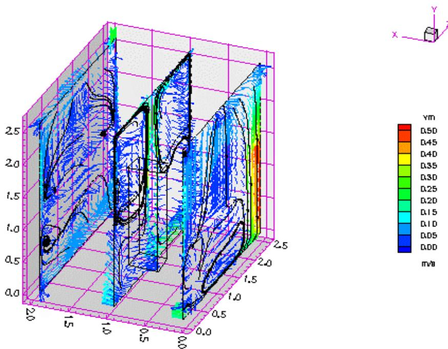
**Fig. 6:** Room air flow with cooled vertical wall surfaces
