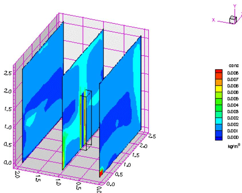
**Fig. 5:** Influence of vertical cooled surfaces on the humidity distribution
