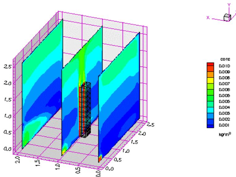
**Fig. 4:** Distribution of air humidity without cooling surfaces
