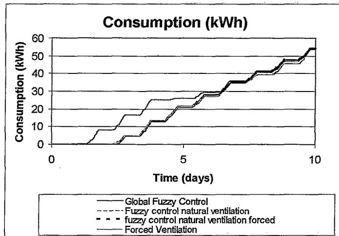
Figure 6. Cumulative consumption levels with set-point 27°C and forced ventilation rate 10 l/s
