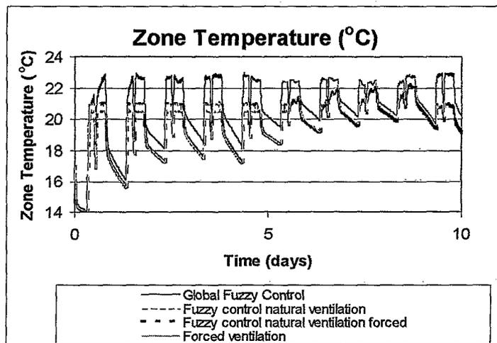
Figure 3. Simulated indoor temperature with set-point 21°C and forced ventilation rate 5 l/s
