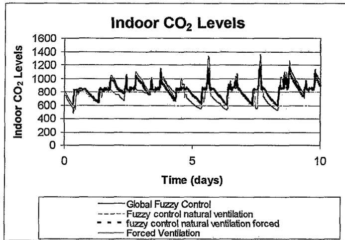
Figure 5. Simulated indoor CO<sub>2</sub> levels with set-point 27°C and forced ventilation rate 10 l/s
