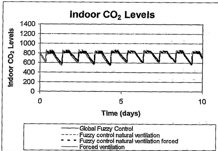
Figure 1. Simulated indoor CO<sub>2</sub> levels with set-point 21°C and forced ventilation rate 5 l/s
