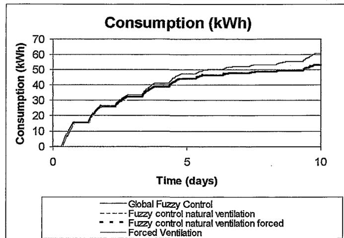
Figure 4. Cumulative consumption levels with set-point 23°C and forced ventilation rate 10 l/s
