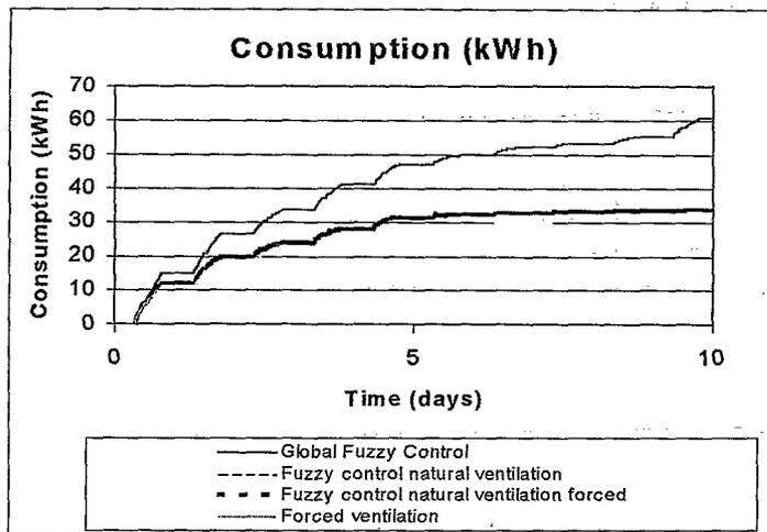
Figure 2. Cumulative consumption levels with set-point 21°C and forced ventilation rate 5 l/s
