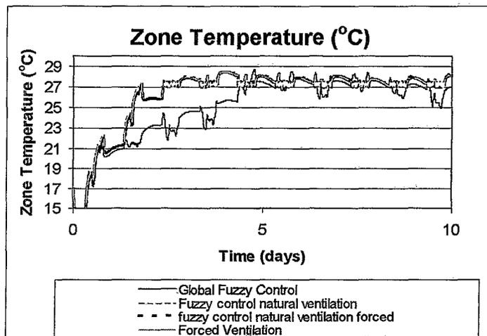
Figure 7. Simulated indoor temperature with set-point 27°C and forced ventilation rate 10 l/s
