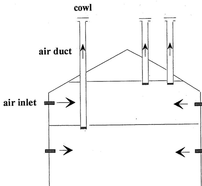
Figure 3 : Passive stack ventilation in a single-family dwelling
