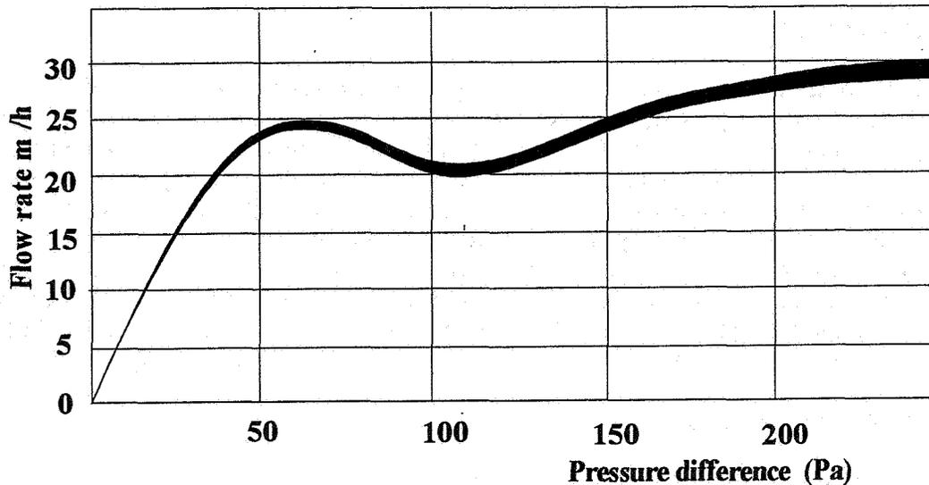
Figure 1 : A characteristic self-regulated air inlet curve.
