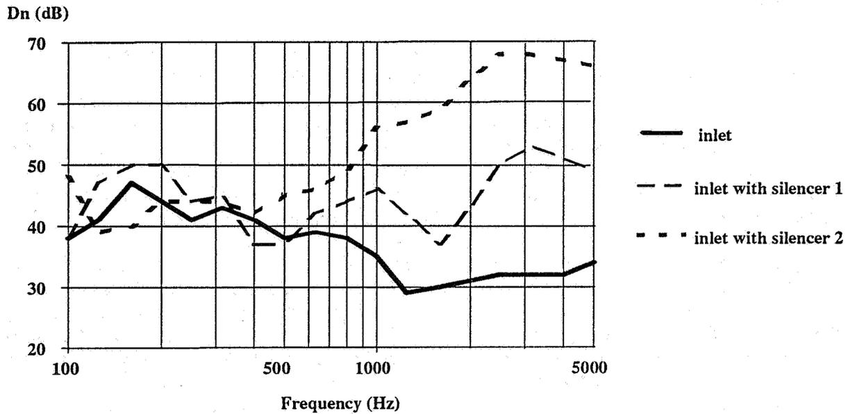
Figure 4: Acoustic attenuation of an air inlet with or without a silencer (the nominal flow rate of the inlet is 30 m<sup>3</sup>/h)
