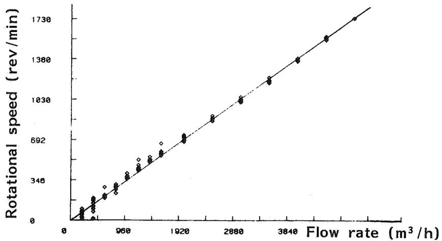
Figure 8. Linear regression analysis. 2-blade impeller prototype (flow rate : 200-5000 m<sup>3</sup>/h,  $\Delta p$  : 0-120Pa), upstream position, combined with Siemens 2CC2 - fan.
