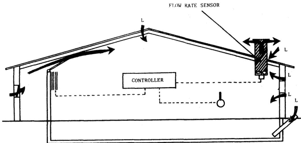
Figure 1. Place where the flow rate sensor should be mounted because of possible leakages in the building envelope (L: Leakage).
