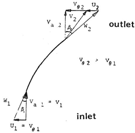
Figure 4. Velocity triangles at inlet and outlet of a turbine blade
