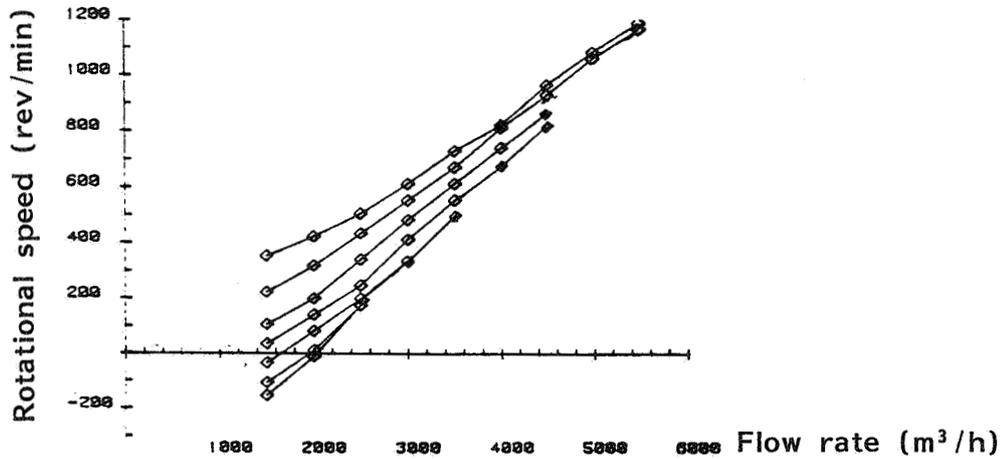
Figure 5b. Rotational speed vs. flow rate for a 2-blade impeller, upstream position.
