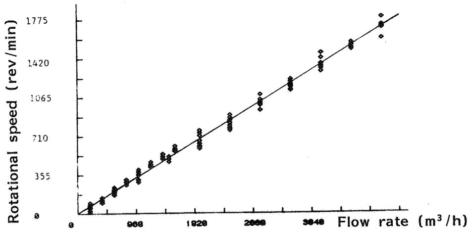
Figure 6. Linear regression analysis. 2-blade impeller prototype (flow rate : 200-5000 m<sup>3</sup>/h,  $\Delta p$  : 0-120Pa), upstream position, combined with Woods 2100-fan.
