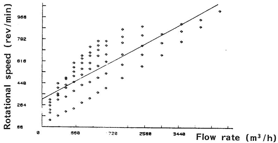
Figure 7. Linear regression analysis. Turbinemeter old design (flow rate : 200-5000 m<sup>3</sup>/h,  $\Delta p$  -120 Pa), downstream position, combined with Woods 2100 - fan.
