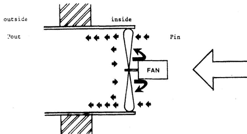
Figure 2. Back flow effect of an axial fan ( $P_{in} \ll P_{out}$ ).
