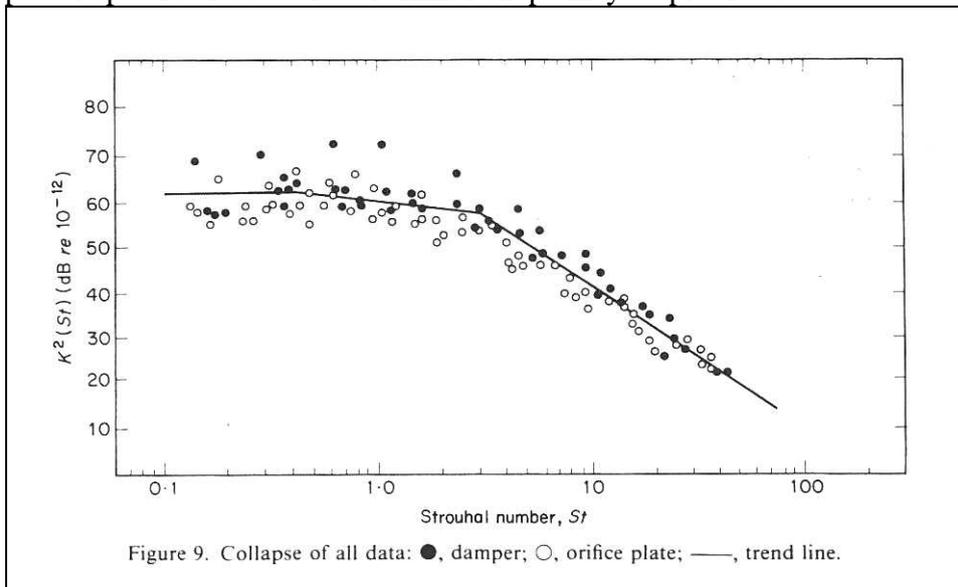
**Figure 10** Function  $20 \log K(St) + 120$  for dampers and orifice plates [7]
