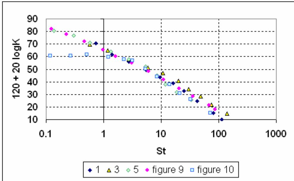
**Figure 12** Function  $20 \log K(St) + 120$  for different geometries of spoilers
