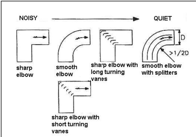
**Figure 1** Guidelines for minimising flow-generated noise in duct bends [1]
