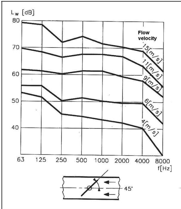
**Figure 5** Flow-generated noise spectra of a damper opened at 45° [1]
