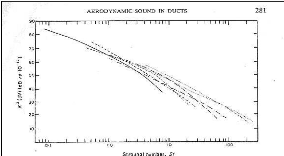
**Figure 9** Function  $20 \log K(St) + 120$  for strip spoilers [6]
