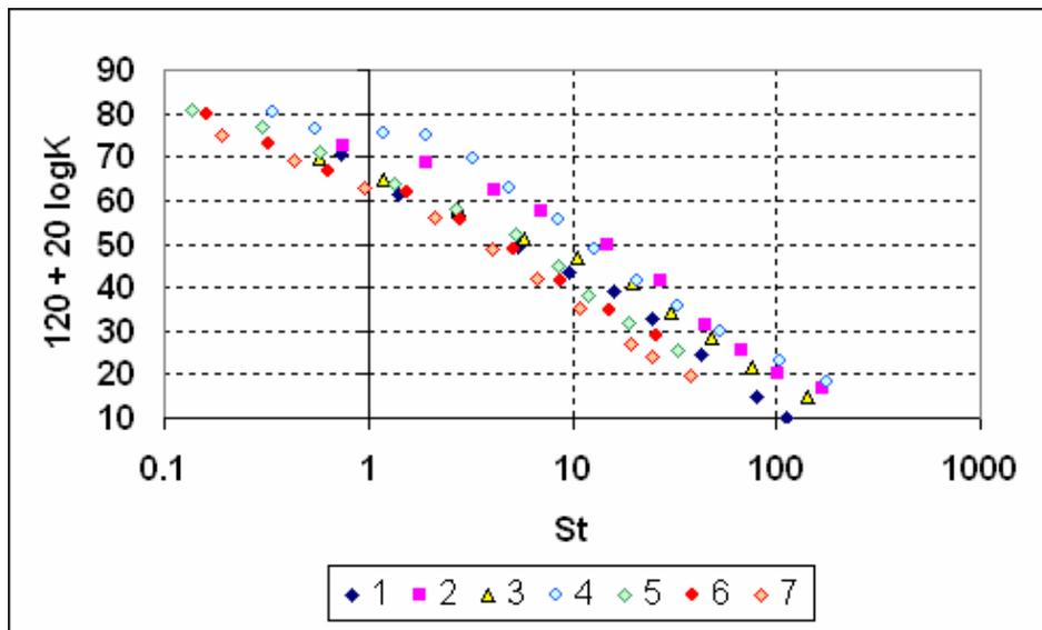
**Figure 11** Function  $20 \log K(St) + 120$  for elbows and branch takeoffs
