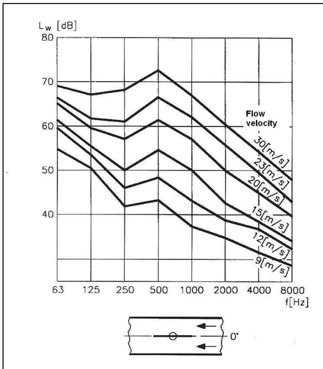
**Figure 3** Flow-generated noise spectra of a wide-open damper [1]
