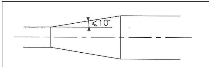
**Figure 2** Gradual transition for limiting flow-generated noise in a duct discontinuity [1]
