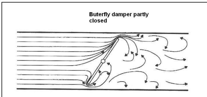
**Figure 4** Flow around a partly closed damper [1]
