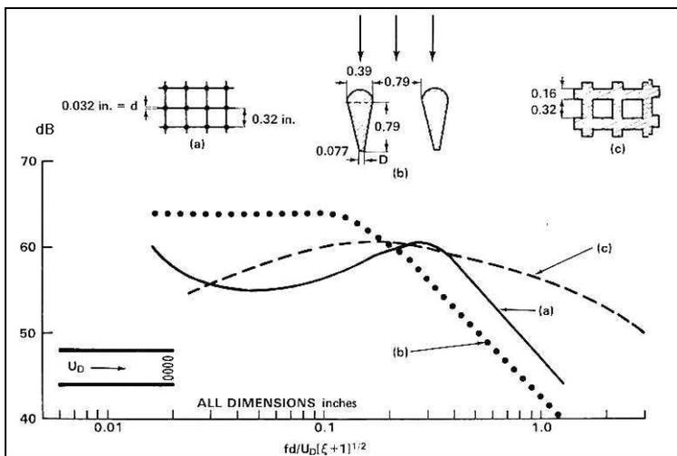
**Figure 6** Function  $F$  for three geometries of gratings [4]
