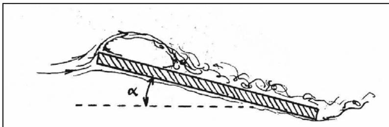
**Figure 10** Flow separation on the leading edge of a flat plate in incidence
