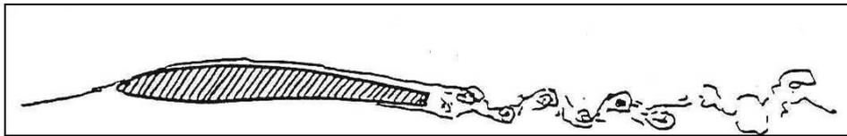
**Figure 11** Vortex shedding in the wake of an airfoil
