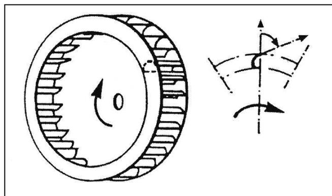
**Figure 6** Centrifugal impeller with forward-curved blades
