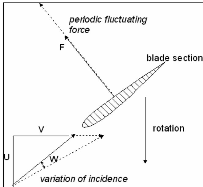
**Figure 9** Velocity triangle at the blade leading edge
