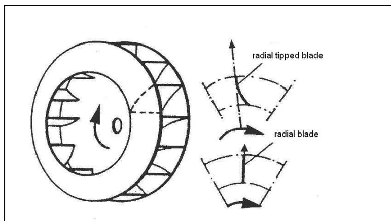
**Figure 5** Centrifugal impeller with radial blades
