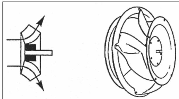
**Figure 7** Impeller of a mixed flow fan
