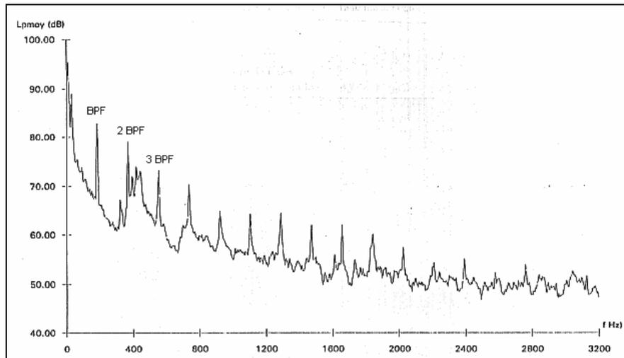
**Figure 1** Example of sound pressure spectrum measured on an axial fan
