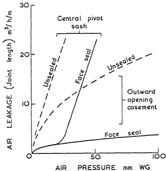
Figure 1 Typical air leakage performance of existing windows
